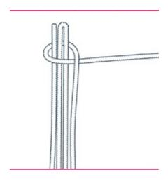
Wrap the long end of the rope around the base of the ropes, weaving it under the outside length and securing the short end in the process.
